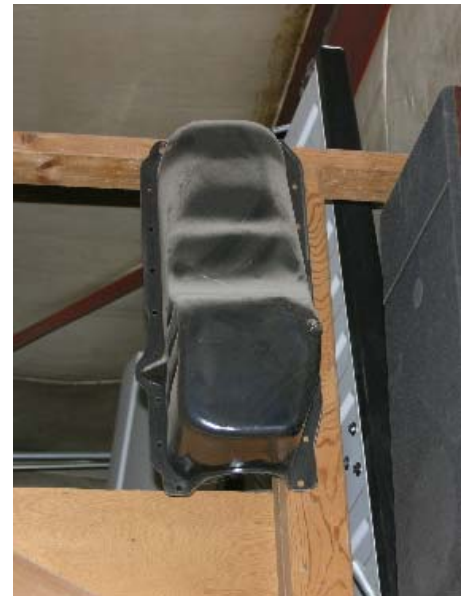
Refurbished oil pan from Police Unit #37, hanging in the shop
