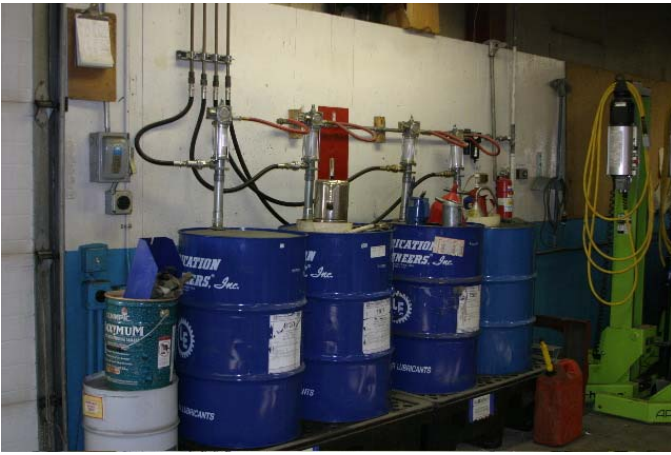
Some of the LE product in the shop, hooked up to overhead dispensers
